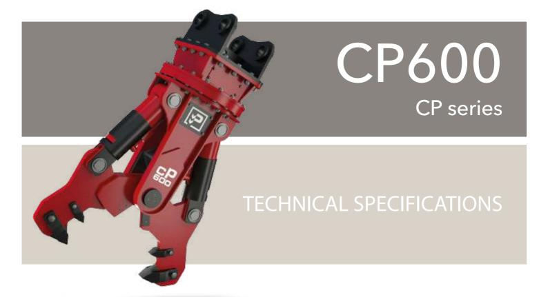
Working weight 620 Kg 5/11 ton Excavator weight Cylinder force 34 t Cylinders working pressure 300 bar 60/120 l/min Cylinder oil flow 100 bar Rotation engine pressure 10/12 l/min Rotation oil flow (Min/Max) Max jaws opening (A) PR 580 mm 300 mm Max jaws opening (A) SC Max jaws opening (A) FR FR Kit (to be mounted on PR jaws) 540 mm Total height (B) 1670 mm hydraulic Rotation 360°
